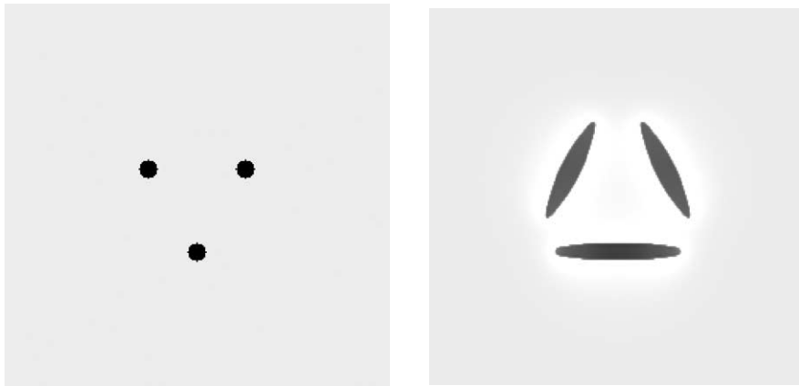
Fig. 2. The shape change of \gamma -hydride sphere particles in the zirconium matrix under the influence of the coherent elastic energy. Each particle was set different initial \eta_p value.
