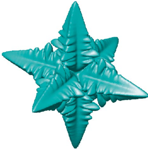
Figure 1 A snapshot of a three-dimensional dendrite in pure Ni with a cubic interfacial energy anisotropy obtained from a phase-field simulation with thermal noises (72) (courtesy of A. Karma). The interfacial energy and mobility anisotropies were obtained from atomistic simulations, and they are matched to the kinetic coefficients in the phase-field model using a thin-interface analysis.
