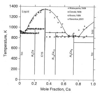
Fig. 3—The Al-Ca phase diagram compared with experimental data.<sup>[3,43–45]</sup>
