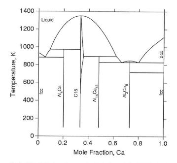
Fig. 1—The Al-Ca phase diagram calculated using only the  $\Delta H (T = 0 \text{ K})$  values in the Gibbs energy description of the nonstable *C*15 compounds.
