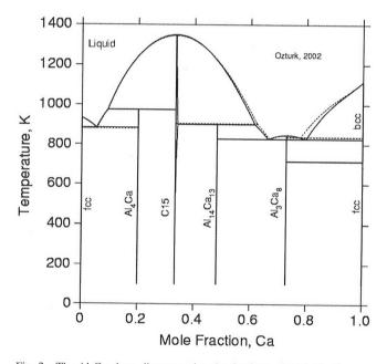
Fig. 2—The Al-Ca phase diagram using the database given in the Appendix. The solid line is the present investigation. The new phase diagram is compared with our previous study (dotted lines).<sup>[1]</sup>
