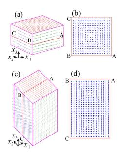
FIG. 1. (Color online) Polarization distributions of  $16 \times 16 \text{ nm}^2$  square nanodots with the thicknesses of [(a) and (b)] 8 nm and [(c) and (d)] 32 nm, respectively, in the  $x_3$  direction. (a) and (c) are the 3D vortex structures; (b) and (d) are the 2D projections of polarizations in the middle planes of the corresponding dots.
