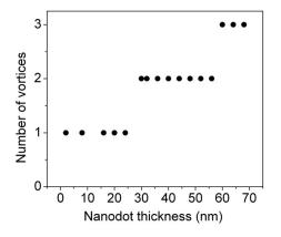
FIG. 2. Number of vortices vs nanodot thickness.
