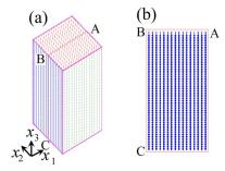
FIG. 3. (Color online) Polarization distribution of a  $16 \times 16$  nm<sup>2</sup> square nanowire. (a) 3D polarization distribution and (b) 2D projection of polarizations in the middle plane of the wire. The periodic boundary condition is used in the  $x_3$  direction for the simulated ferroelectric nanowire.
